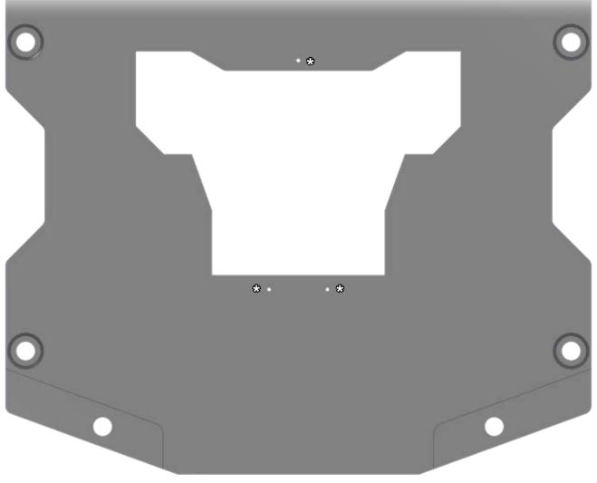
\*holes must be drilled out large enough to accept Ø1/4" hardware.
