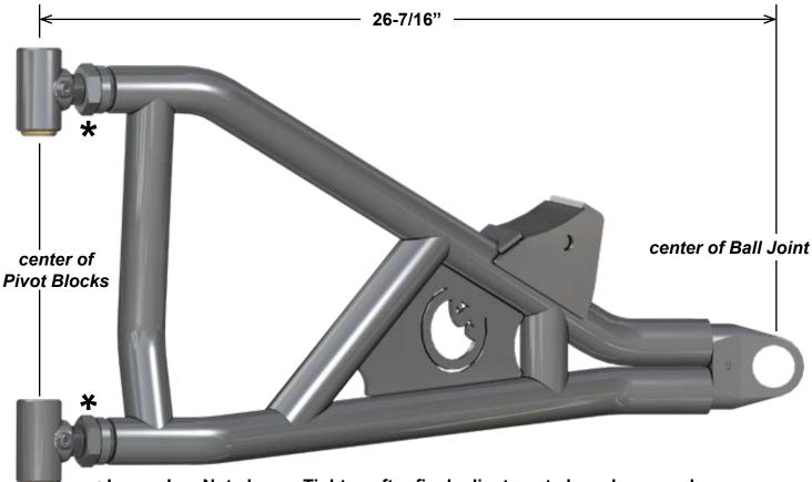
\*Leave Jam Nuts loose. Tighten after final adjustments have been made.
