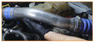
6. Disconnect the air temperature sensor from the cold-side pipe.
