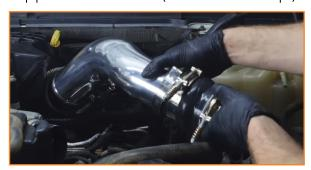
18. Connect the open end of the straight hot-side coupler to the intercooler.(1x 79/87 T-bolt clamps)
