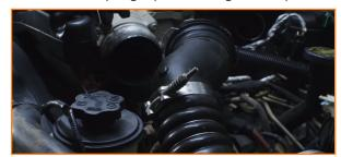
8. Compress the clamp on the small hose connected to your intercooler, and then slide the hose off the port. (1x spring clamp)
