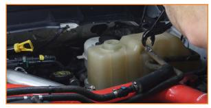
3. Detach the quick-disconnect above the upper radiator hose. Press the blue tab at the center and pull the quick-disconnect off the port.
