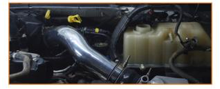
19. Attach the large coupler with a bend to your cold-side pipe, specifically on the end farthest from the sensor. (1x 79/87 T-bolt clamp)
