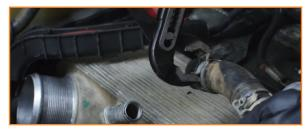
9. Release the quick-disconnect from the intercooler. Pinch the tabs and pull the connection off the port.
