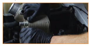
13. Transfer the grommets, spacers, and hardware from the stock intercooler to the Mishimoto intercooler. There is one on top of the intercooler, on the port, to allow for the quick-disconnect to attach. There are two grommets on the sides and a spacer at the bottom on the back of the intercooler.
