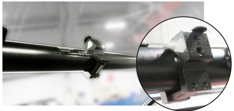
Install both Front and both Rear locations first. You will then install the Center Clamp and 4 side brackets in the following steps.
