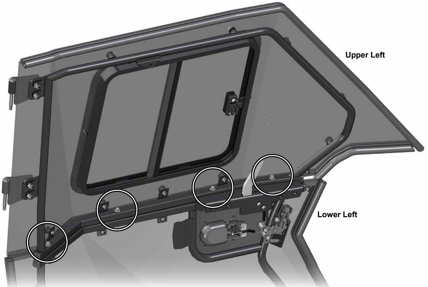
**SuperATV Roof:** Place assembly and SuperATV Roof onto machine. Secure with hardware shown; do not tighten.
