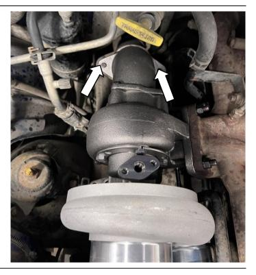
3. Connect the turbo to the downpipe using a 13mm socket.
