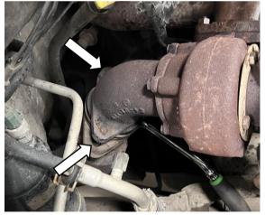
7. Remove the four turbo mounting nuts with a 15mm socket/wrench.
