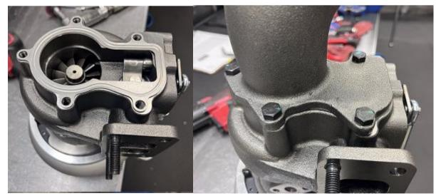
Using the new gaskets (FT-920156020 & 3922794) provided in the kit, install the oil supply fitting from the old turbo to the Screamer turbo.Tighten fitting to 36 N.m (27 ft.lbs) with a 19mm socket.
