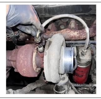
5. Remove the turbo outlet elbow from the turbo by removing the Tbolt clamp and V-band clamp using a 10mm and 11mm socket.
