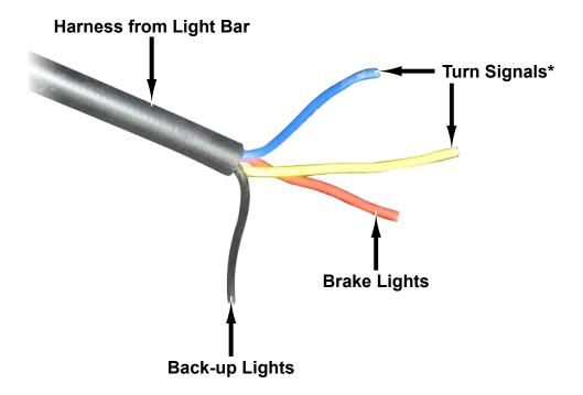
\*Right or Left Turn Signal will depend on Light Bar mounting orientation.
