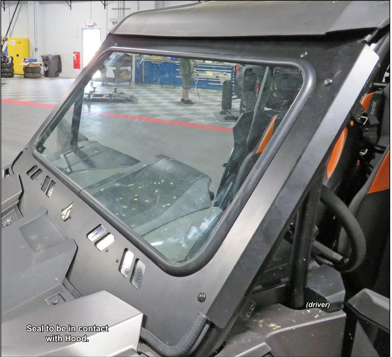
Secure Windshield to Clamps with hardware shown.
