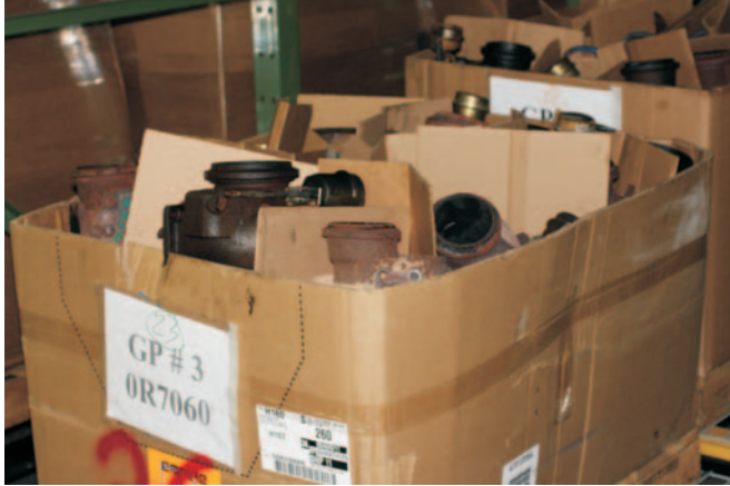
Pack core in original box or add cardboard dividers if necessary to prevent damage in-transit
