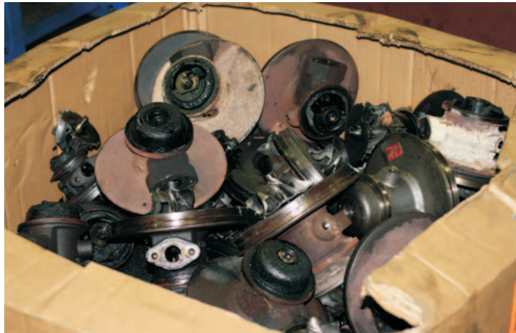
Cores were not segregated and were incomplete. Cores received additional damage as a result of packaging negligence
