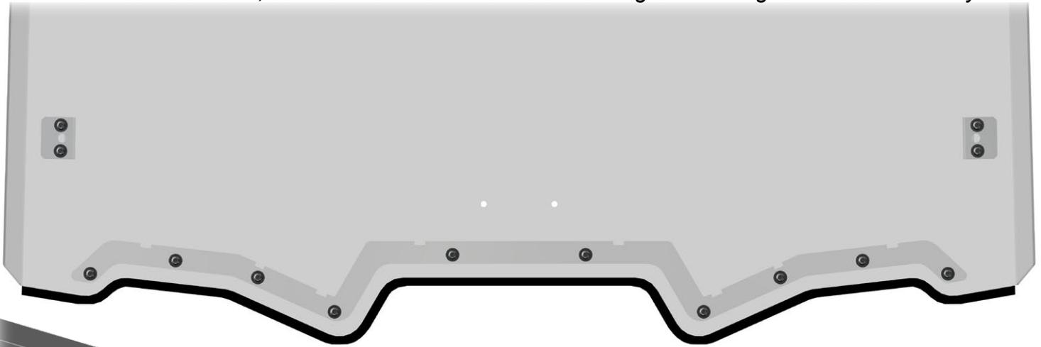
Install Bulb Seal bottom of Windshield as shown.
