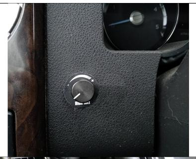
If mounting in the knee bolster, be aware of the reinforcement plate behind the bolster which will limit the available spaces to mount the switch.
