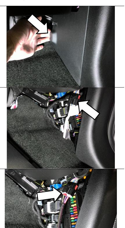
Plug in the BD High Idle wiring harness to this connector.
