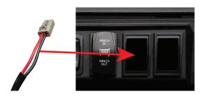
1. Locate an empty switch knock out in your machine. Then push the wire harness from the inside of your machine through the empty knock out until the switch snaps into place.
