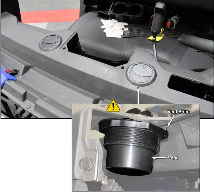
**DRIVER SIDE ONLY:** Vent Shim must be installed between nut, on Vent, and Dash; tighten.
