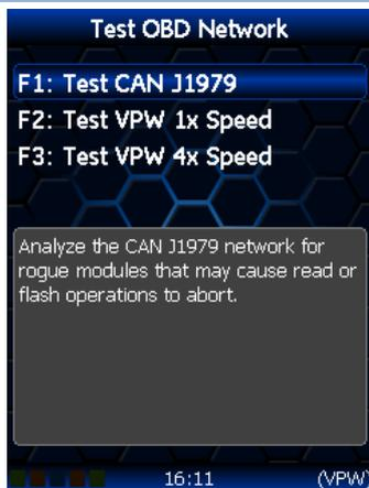
F1: Test CAN J1979; Analyze the CAN J1979 network for rogue modules that may cause read or flash operations to abort.
