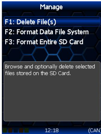
F1: Delete File(s); Display and optionally delete files stored on the SD Card.
