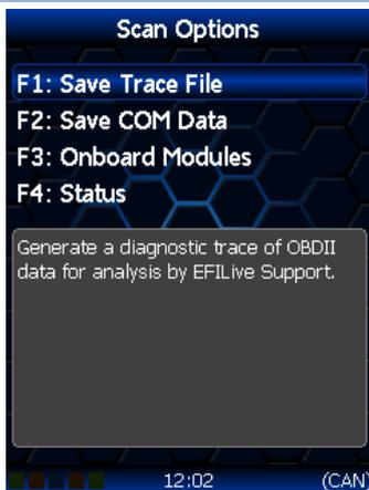
F1: Save Trace File; Generate a diagnostic trace of OBDII data for analysis by EFILive Support.
