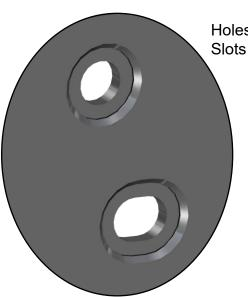
Holes = Installer must drill pilot hole. Use provided self tapping hardware. Slots = Stock mounting locations. Use provided threaded hardware. - Install Rear (B) to stock mounting locations with hardware shown.
