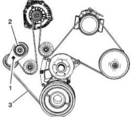
Remount A/C compressor and install serpentine belt.
