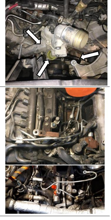
Carefully bend return line in valley to be parallel to machined surface of L/H intake manifold. This may need further adjusting later once new pump is installed.
