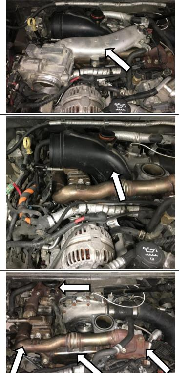
Remove aluminum intake with throttle body and support bracket.
