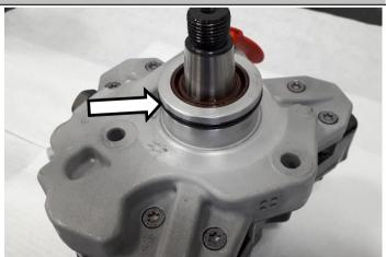
Install pump mount adapter **1500780** onto pump, and tighten three mounting bolts **FT-11116059** to **18 ft-lbs**.
