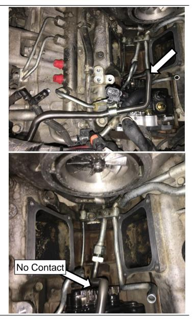
Install high-pressure line **1500775** from CP3 to R/H fuel rail, and install fuel rail plug **1500778** as shown.
