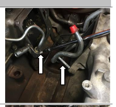
If necessary, adjust crossover and return lines to not contact CP3.
