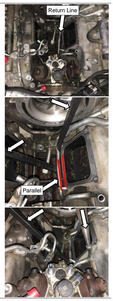
Remove CP4 from cylinder block, and polish mounting bore to aid CP3 installation.
