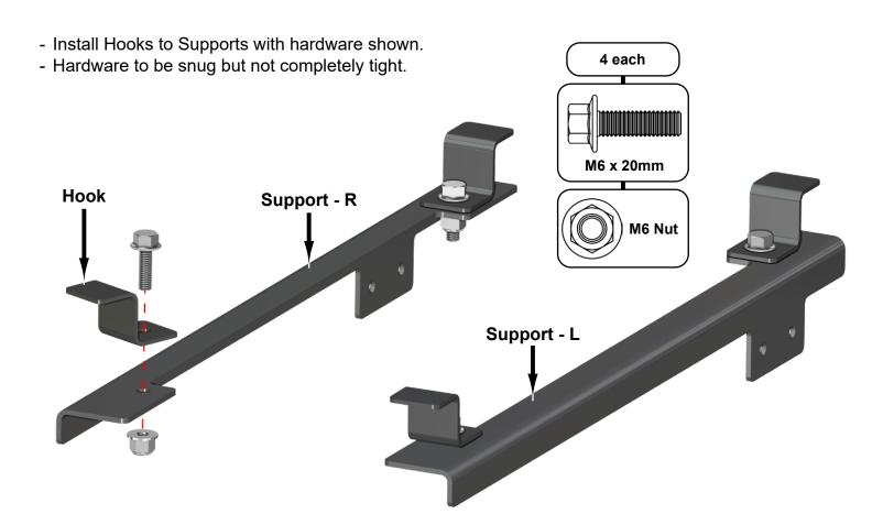
Place Supports into machine in locations shown.Secure Heater to Supports with hardware shown.
