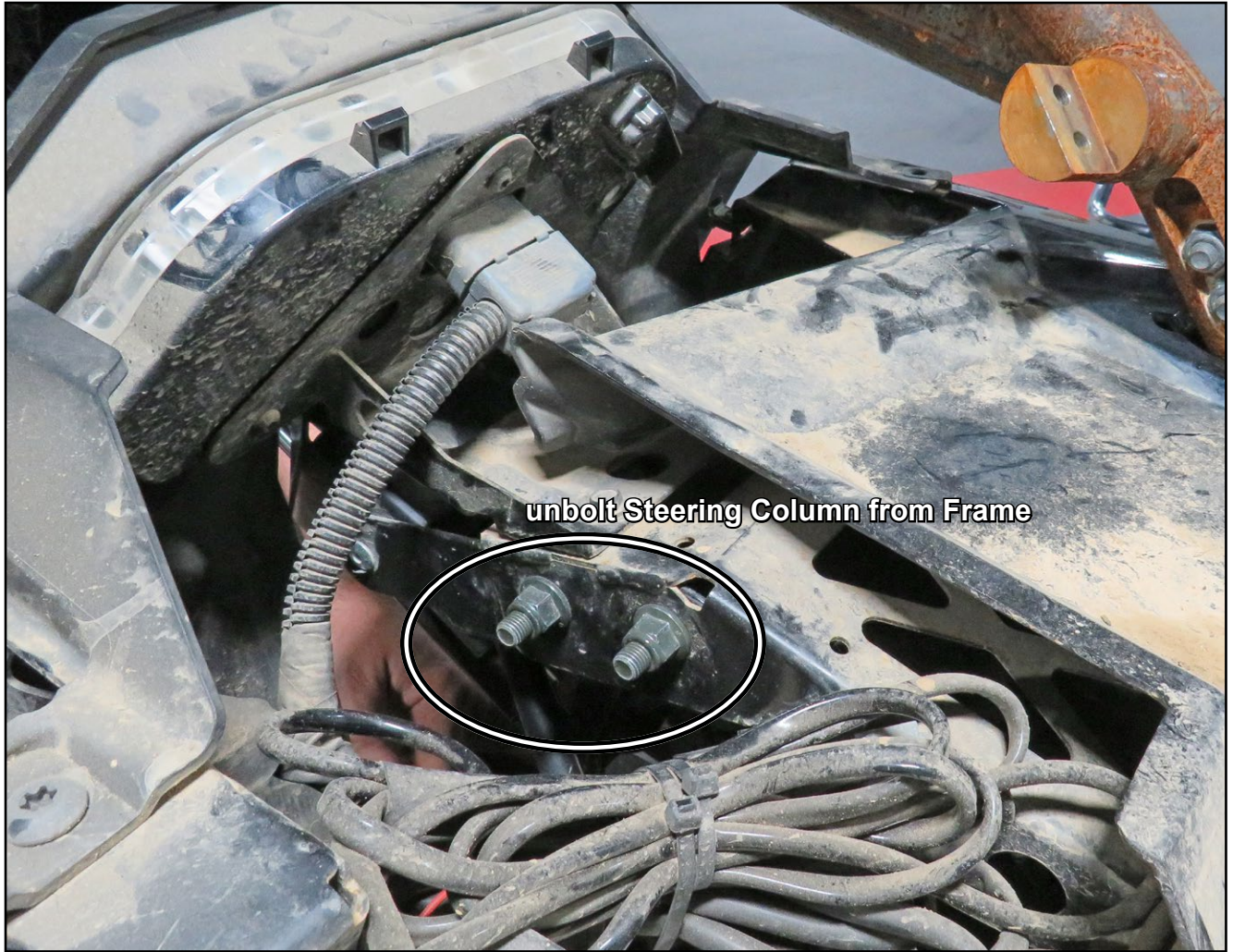
remove Steering Column and Upper Shaft from machine
