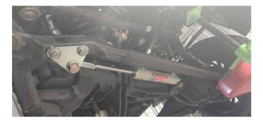
**13)** Using the (2) factory bolts, install the tie-rod mount bracket as shown above. Bolts need to be installed from the bottom up and secured with the factory nuts. The shaft side of the cylinder will be installed using this bracket and supplied hardware.
