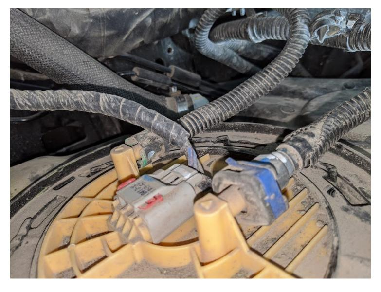
Reconnect the feed line, return line and electrical connector. Make sure the connectors are locked. To make sure they are locked, gently pull on the connectors to make sure they won't come off and are locked in.
