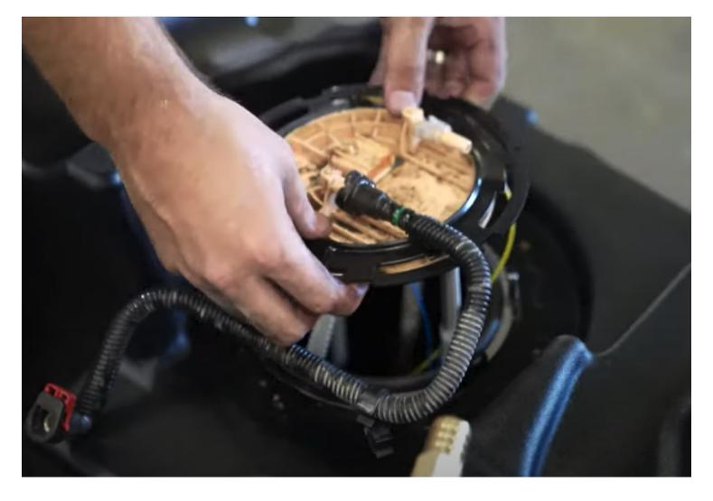
Drop in the OEM sending unit into the S&B Tank. The retaining ring included with the tank will be used.
