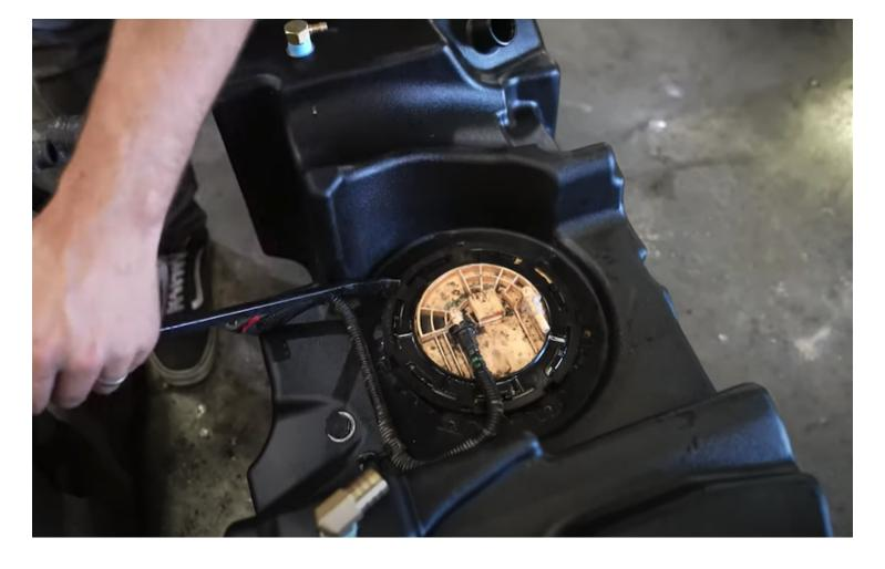
Place the included locking ring over the sending unit flange. First, by pressing down on the ring, get the ring started under the teeth on the tank. Once started, hit the ring clockwise until it passes under the indentation on tank teeth
