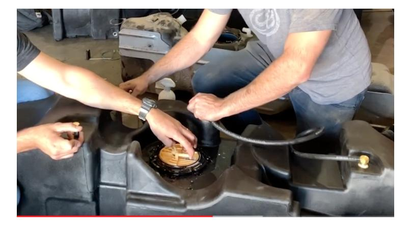
Poke a small hole in the rubber cap covering the filler spout on the S&B Tank, block off the openings in the tank with electrical tape or cover with fingers, spray the sending unit o'ring area with soapy water and pressure test the tank to make sure the o'ring was properly seated and there are no leaks in the tank.
