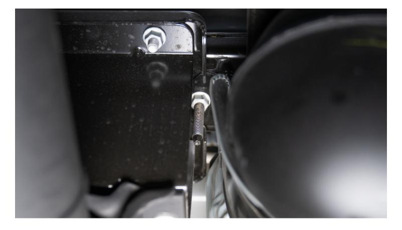
If you are working with the truck on a lift place a jack centered under the tank. Remove the OEM fuel tank straps. These are 16mm nuts that hold the straps to the studs. When removing the straps from the frame side, you will need to push the strap up to release the strap from the cradle.
