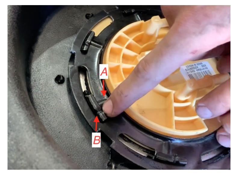
Ensure the locking ring is fully rotated until the rib on the OEM locking ring(point A) is PAST the indentation on the S&B receiving ring(point B).
