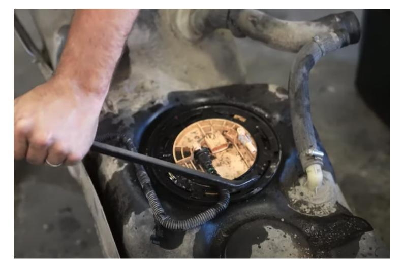
After the tank has been dropped. Remove the OEM fuel sending unit locking ring from the tank by hitting the ring counterclockwise. The OEM o'ring won't be used again.
