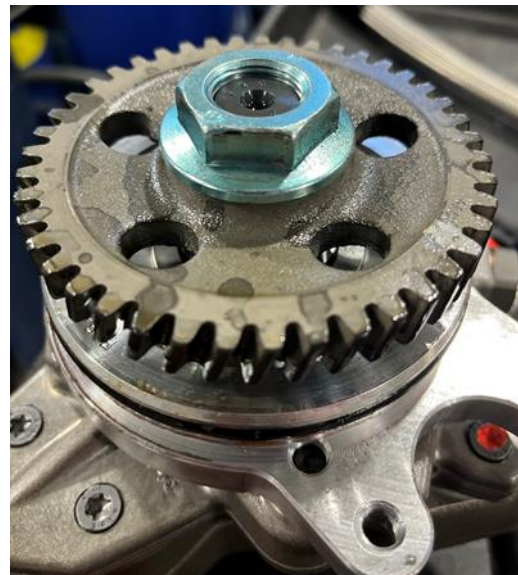
Fig. 12: Install the CP4 nut onto the CP3
