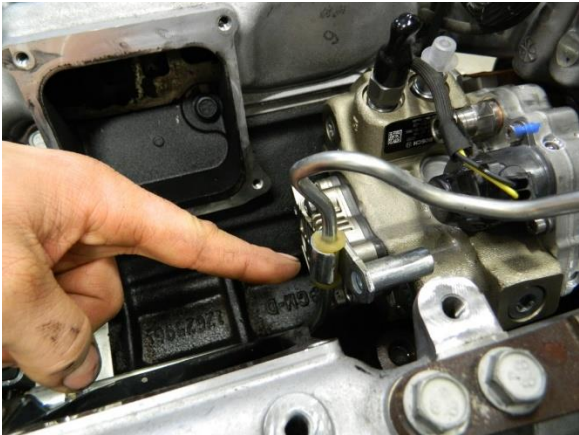
Carefully remove high pressure line bracket
