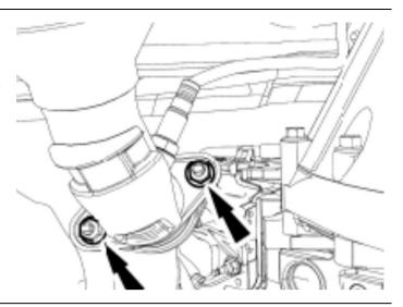
Install the RH turbo outlet pipe to the turbo and attach it to the mounting bracket.
