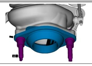
Install the new turbo gasket onto the turbo flange.
