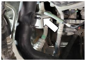
First, Lay RH turbo outlet tube into place
