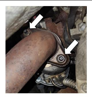
With the exhaust disconnected, adjust the exhaust rearward to ensure clearance between the turbocharger flanges and the downpipes.
