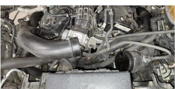
Disconnect the PCV pressure sensor electric connector, PCV tube quick connect couplings and remove the PCV tube.
