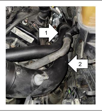
Connect the PCV pressure sensor electric connector, PCV tube quick connect couplings and install the PCV tube.
