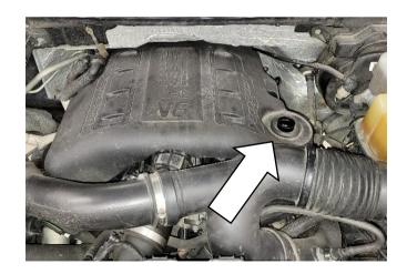
Disconnect the MAF sensor in the intake pipe.
