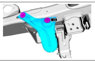
Reinstall the starter and trans cooler line support into the transmission.
