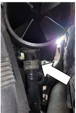
Loosen the clamps on the pipes which mount to the turbocharger and gently remove hose from the compressor cover.
