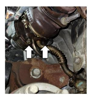
Install the oil return tube bolt at the cylinder block.
