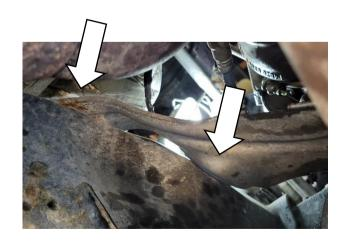
Remove the retaining clip in the coolant fitting on the top of the turbo and disconnect the coolant supply tube at the turbocharger.
