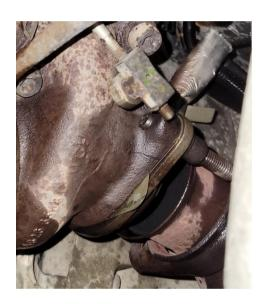
On the driver side of the frame, remove the 2 heat shield bolts and the heat shield.
