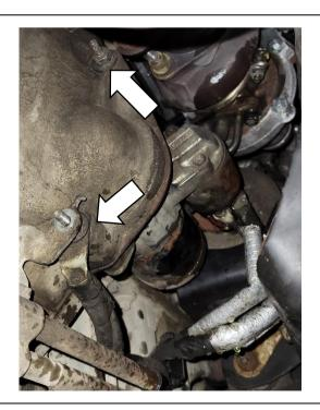
Remove and discard the 2 catalytic converter-to-turbocharger mounting flange nuts on both sides of the vehicle.
