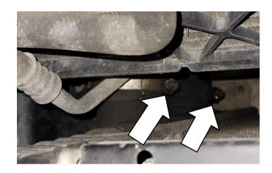
Release the turbo inlet & outlet tube from the bracket grommet and remove the inlet & outlet tube.
