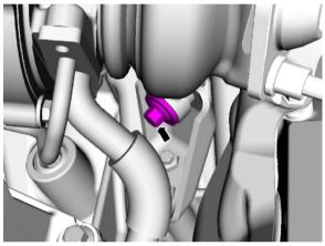
Remove the retaining clip on the coolant fitting on the inside turbo. Disconnect the coolant return tube at the turbo. Remove the 3 turbo mounting bolts and the turbo.
