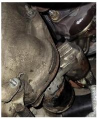
Slide exhaust forward into position.
