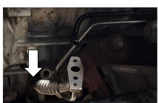
Install the new turbocharger oil inlet gasket.
