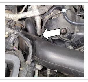
Connect the turbo inlet pipe hose to the RH inlet pipe.
