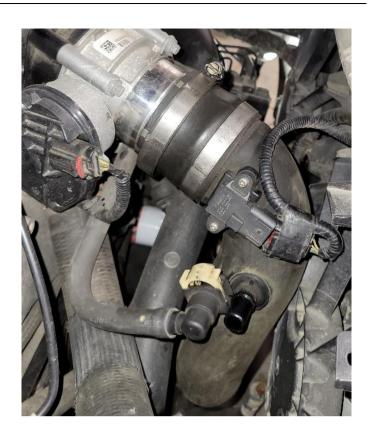
Disconnect the vacuum line from the passenger side turbocharger outlet pipe and remove the pipe.
