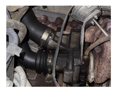
Loosen the intercooler to inlet pipe clamps located between front bumper and radiator.
