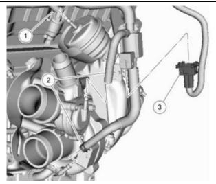
Connect the upper coolant supply tubes with retaining clips.
