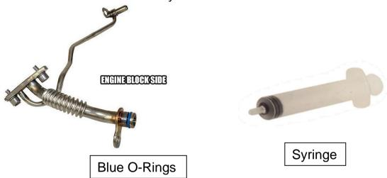
The provided blue O-rings are intended for the oil drain tube, while it is not necessary to replace this part, stock OEM O-rings can leak, and we have provided this part if you wish to replace the O-ring while installing this kit.
