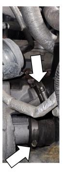
Install the Upper Air Cleaner lid and Y-Pipe to the turbo inlet pipes. Tighten all intake connections. Connect MAF sensor to harness.
