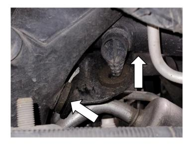
Disconnect the boost sensor and disconnect the pipe from the throttle valve and remove to allow for removal of the driver side turbocharger outlet pipe.
