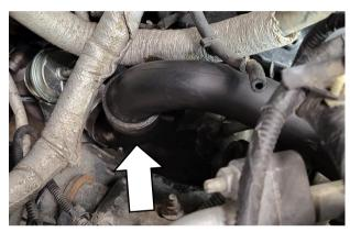
Install the RH turbo inlet pipe to the turbo and attach it to the mounting bracket.
