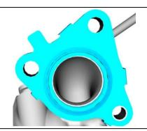
Install new oil return tube o-ring and install the oil return tube assembly. Reinstall retaining clips.
