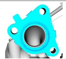
Remove the 2x turbo exhaust flange stud bolts and exhaust flange.
