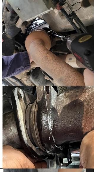
To gain more space for removal of the manifold remove the mid-pipe exhaust hanger as shown.
