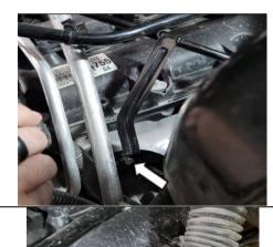
Align the previously created marking and insert the upper steering shaft into lower and tighten the bolt.
