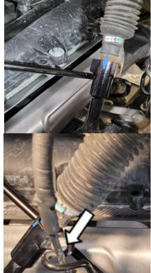
Check oil dipstick-for clearance against the hard lines after it was relocated.
