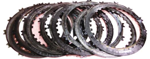
Burnt clutches are not covered by warranty. Failure to correctly adhere to this procedure may result in clutches that look like this.
