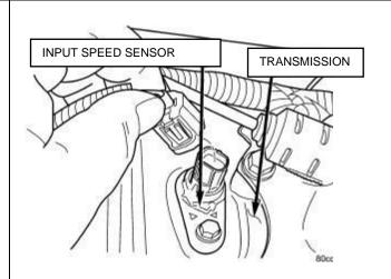
Disengage the transmission solenoid/TRS assembly connector from the transmission solenoid/TRS assembly.
