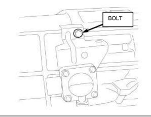
Disconnect gearshift cable from transmission manual valve lever.
