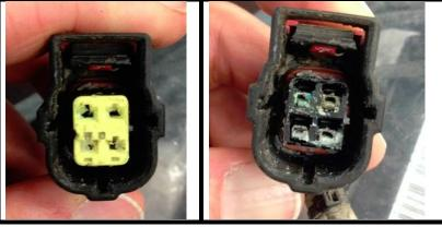
Corroded line pressure sensor connections are known to cause erratic shift quality concerns due to wildly varying transmission line pressure and in some cases cause broken transmission shafts. If corrosion is present, replace the entire connector assembly.
