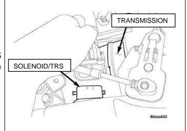
Disengage the line pressure sensor connector from the line pressure sensor. Thoroughly inspect both sides of the connector for corrosion or debris. This has been a known issue and can cause severe damage to the transmission if not corrected.
