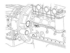
Disengage the output speed sensor connector from the output speed sensor.
