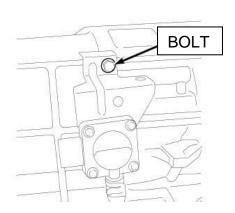
Connect cooler lines to transmission.
