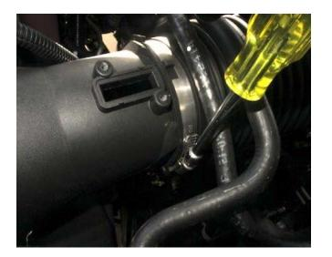
Once the hose clamp is loose, pull tube to the right to remove from factory airbox cover.
