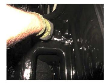
Install the Air Filter (E) by pressing the filter tabs through the side of the Airbox (A). The filter should lock into place when the tabs are secured.
