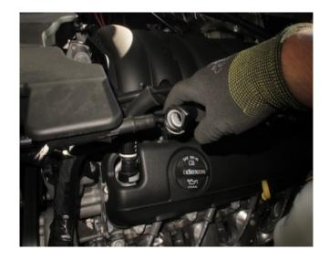
**STEP 7** Loosen the hose clamp at the throttle body.
