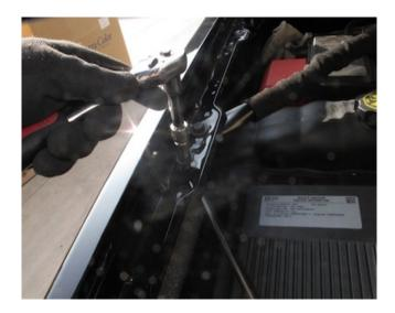
Reconnect the negative terminal on both batteries. Inspect your installation, make sure the kit is properly positioned and all fasteners are secure. Affix the ID label near the intake kit. The installation is now complete.
