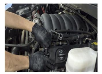
Remove the top bolt from the front cross bar using a 10mm socket.
