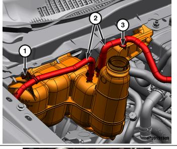
12. Cut the cable ties (1, 2) securing the NOx sensor wire harness, actuator harness, and turbo speed sensor harness.
