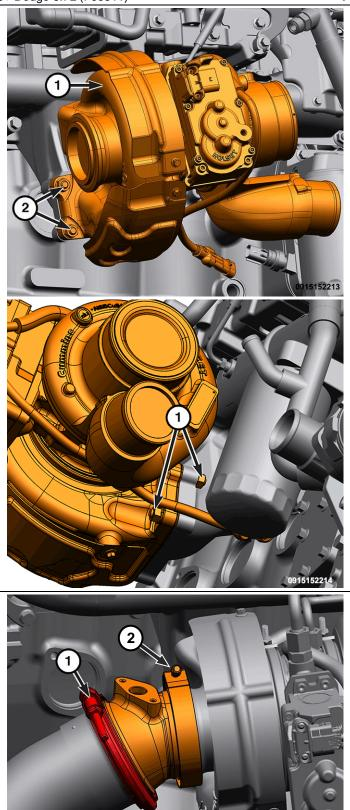
Install the exhaust isolator (2) and the transmission oil cooler line bracket to the transmission and tighten the bolts (1, 3) to 24 Nm (18 ft-lbs).
