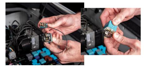
STEP 4: Reinstall the two relays back into their original location. Route the connecting wire along the side of the relay box. Install the relay panel cover.
