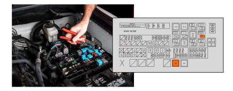
STEP 3: Insert the two relays that were removed through the All Lights On boards with the wire connection facing towards the top of the relay. The board will make a firm connection with the relay.
