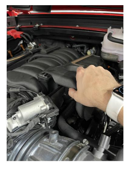
The engine cover is held in place by 2 rubber grommets, firmly lift up on the cover to pop it out of place.
