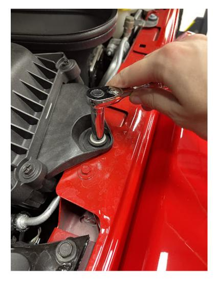
With the engine turned off and cooled down, unscrew the bolt securing the stock airbox on the driver's side with a 10mm socket or wrench. Set the bolt aside it will be reused later to install the S&B airbox.
