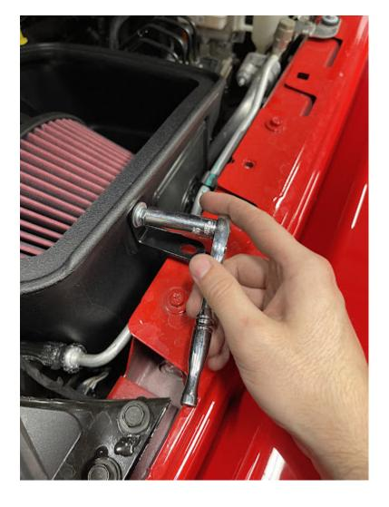
First, install the short side of the angle bracket onto S&B airbox with bolt, washer, and lock nut. Place rubber washer underneath the bracket against the painted side to protect from scratches and reinstall stock bolt into the fender using 10mm socket or wrench.
