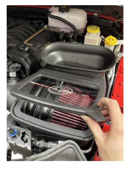
Remove the protective wrapping off the polycarbonate lid. Install the snap-in silicone lid seal around the polycarbonate lid. Slide S&B snap-in lid to backside of airbox first and then apply pressure around the perimeter to lock it into place.
