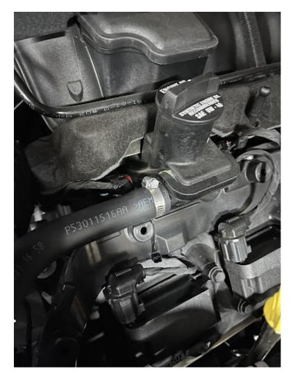
Slide both hose clamps onto CCV hose and tighten using  $\frac{1}{4}$ " wrench or flat head screwdriver onto S&B tube and engine.
