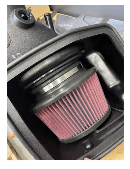
First, place S&B filter in airbox and make sure hose clamp is loose, then push tube through tube seal and directly into filter, tighten hose clamp with 5/16" wrench or flat head screwdriver.
