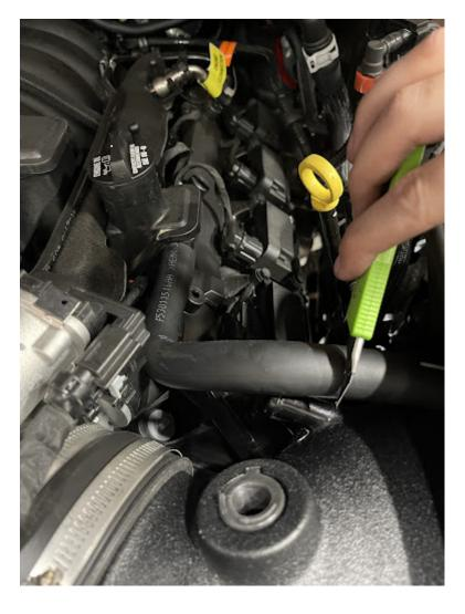
Slide the CCV hose back onto the engine first and then line up the hose with the nipple on the S&B tube. Use a knife or scissors to cut 2-3 inches off the stock CCV hose so that it slides all the way over the nipple on the tube without the hose collapsing in on itself.
