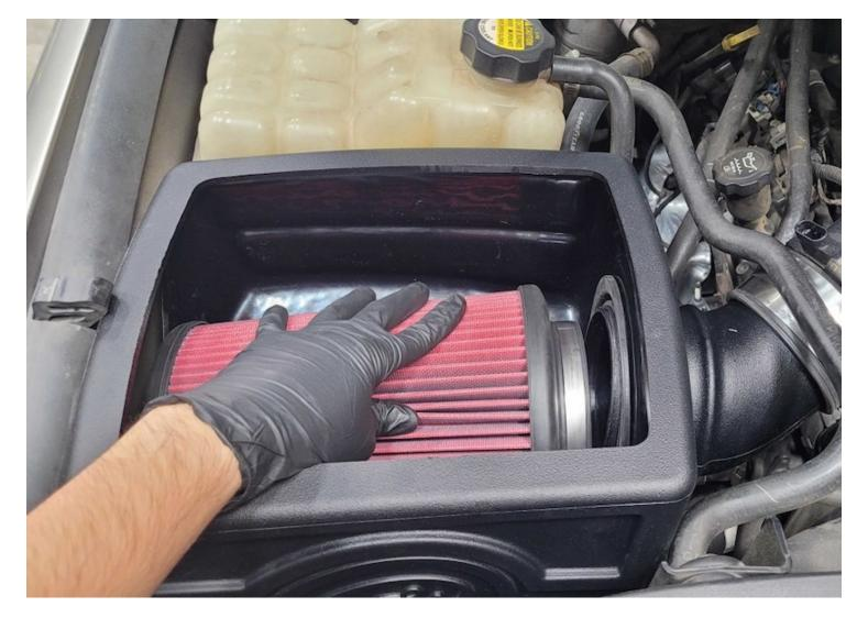
Install the S&B Air Filter (c) and #72 Hose Clamp (D) onto the Filter to MAF Tube (J or Q). Insert the Filter to MAF Tube(J or Q) fully into the S&B Air Filter (c) until it stops on the Filter flange shoulder. The Filter flange should line up with the bead on the tube.
