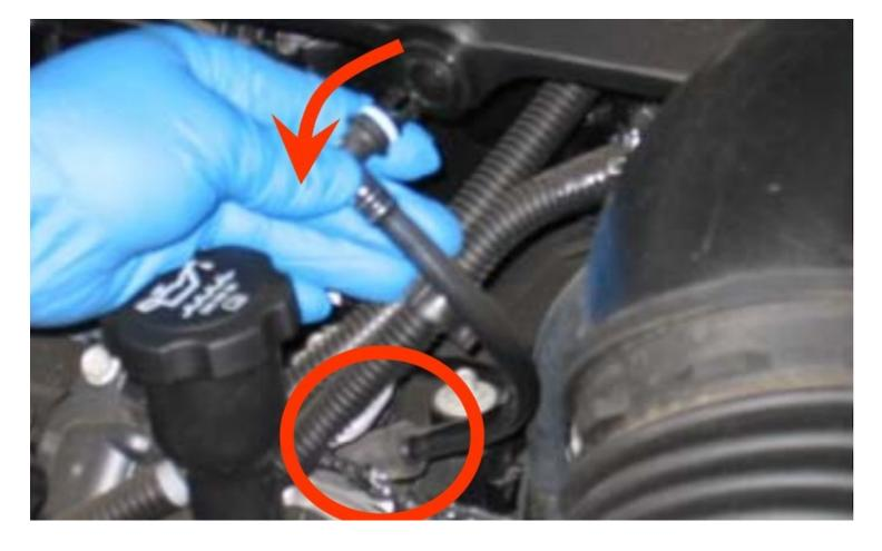
If equipped, pull the crankcase vent line from the OE tube and then from the engine along with the rubber connector and remove it from the vehicle.
