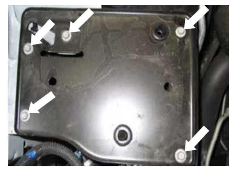
Remove the OE tray from the vehicle. Four of these bolts (if long enough), can be used to secure the S&B airbox to the vehicle. IF too short, then use the supplied Allen head screws (H) and ss washers (G).
