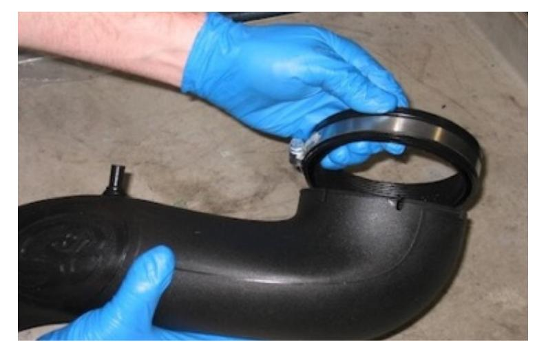
Slide the Silicone Coupler (N) over the Intake Tube (M) throttle location along with the #73 Hose Clamp (D), do not fully tighten at this time.
