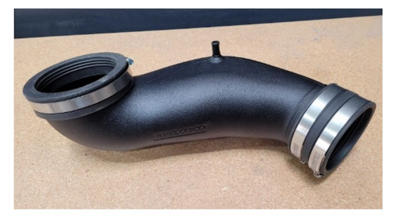
Slide the Straight Coupler (L) over the Intake Tube (M) MAF sensor location along with the #50 Hose Clamp (K), do not fully tighten at this time.
