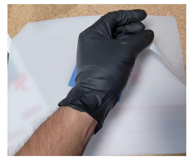
Peel off the protective covering on the Polycarbonate Lid (A). Do not forget to remove the protective covering around the S&B logo.
