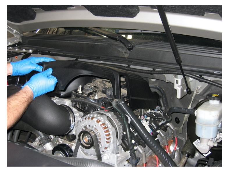
If equipped: Loosen the retaining bolt and pull up and out to remove the engine cover from the Vehicle.
