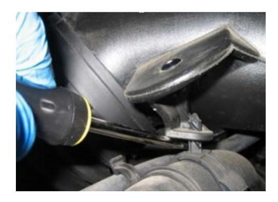
Carefully pry the hose router clamp from the OE air intake tube.
