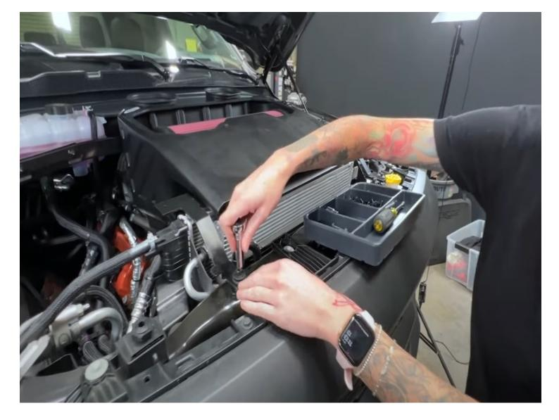
Install the front S&B airbox bracket hardware using a T27 Torx bit and driver or 10mm socket. After all support brackets are secured, tighten the 4 M6 screws and nuts from Step 21.
