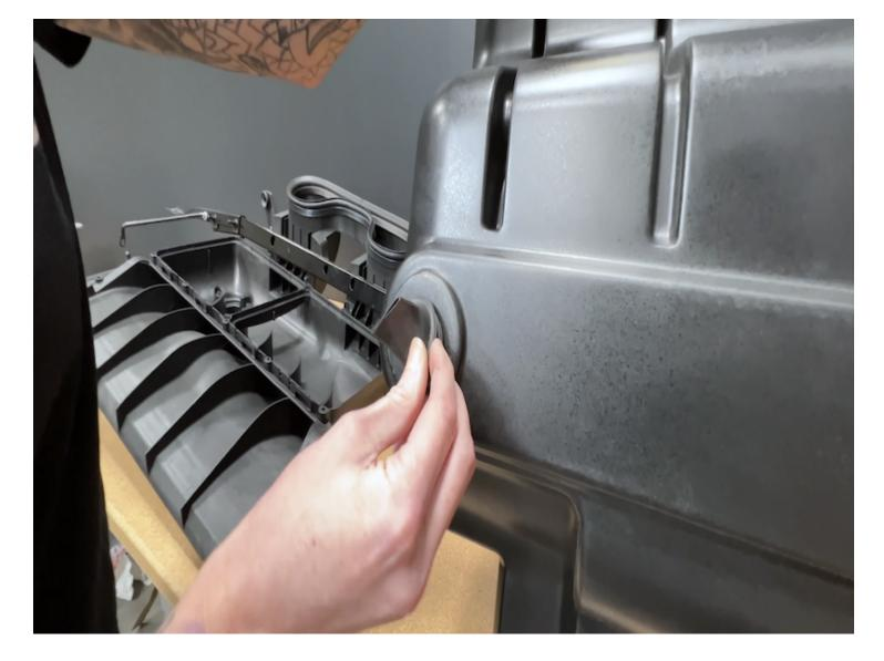
Install the silicone one-way valve onto the bottom of the airbox
