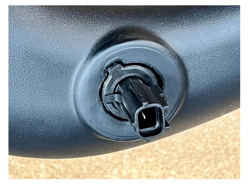
Install the S&B IAT Sensor grommet onto the S&B intake tube. Transfer the IAT sensor from the OEM tube into the S&B tube as shown. The locking tab should rotate over the ramp and lock into position, use the turn arrow for indication.
