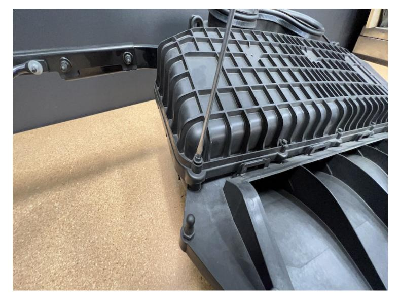
Remove the hardware securing the airbox to gain access to the bracket mounting hardware using a long reach flathead or Phillips head screwdriver. 10 locations in total.
