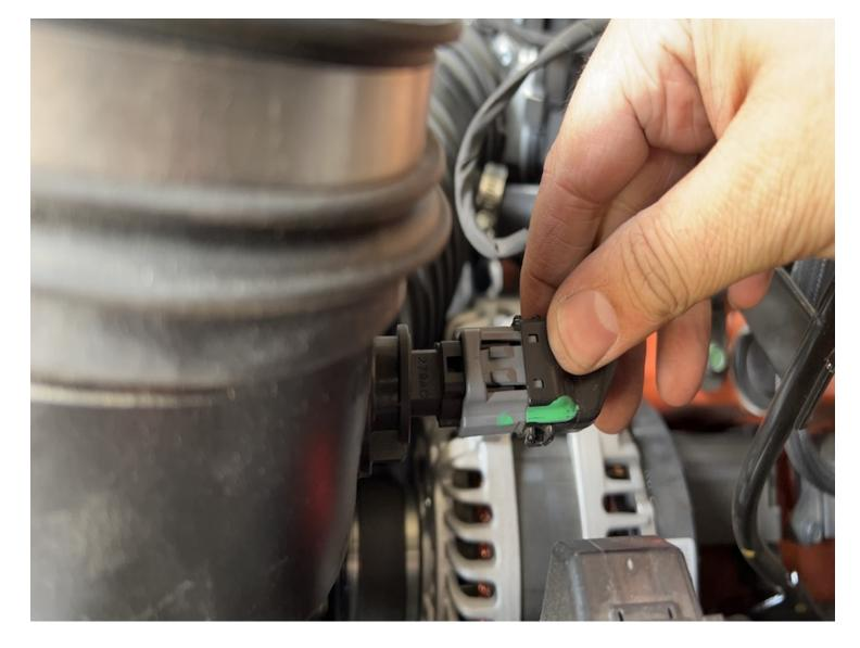
At the tube, unplug the IAT sensor harness from the stock sensor connection.
