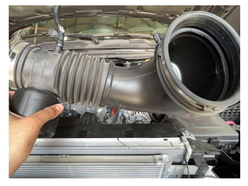
Loosen the hose clamp at the throttle body and disconnect the intake tube. Pull the tube assembly out of the engine compartment and set it aside.
