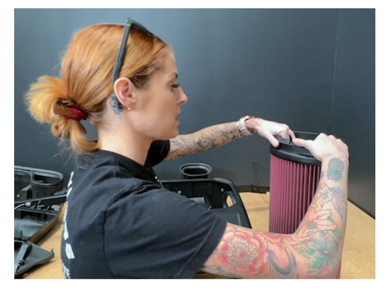
Install the S&B snap-in filter into the airbox. For easier installation, fold the filter flange inward towards the inside of the filter. Once the filter is in the airbox push the snap in a portion of the flange through the opening of the airbox. After the filter is snapped into place, fold the flange to its original position.
