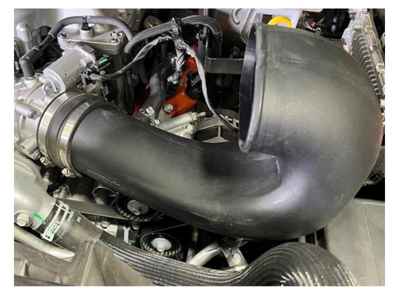
Install the tube into the vehicle by pushing the coupler over the throttle body. Push the CCV tube over the CCV connection end, and rotate into position as needed. Be aware to allow the fuse box clearance to be removed easily for future access. Tighten the hose clamps.
