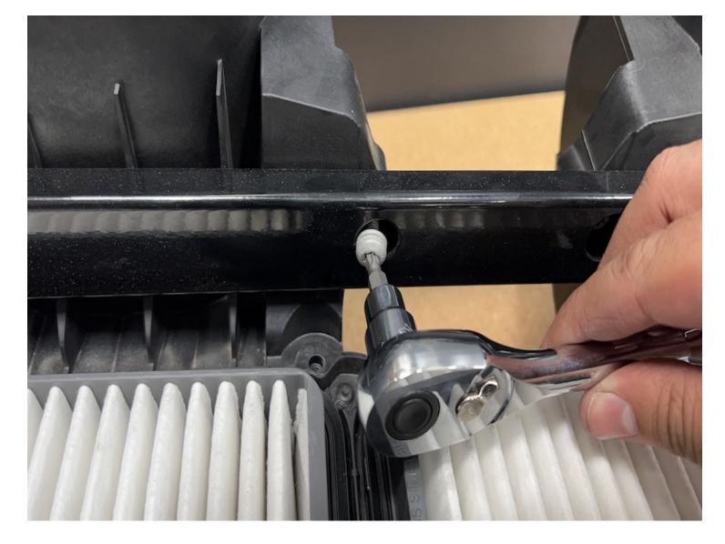
Remove the 4 airbox bracket mounting screws using a T27 Torx bit and driver. Separate the stock airbox from the mounting bracket support. Set the support bracket to the side to be reused.
