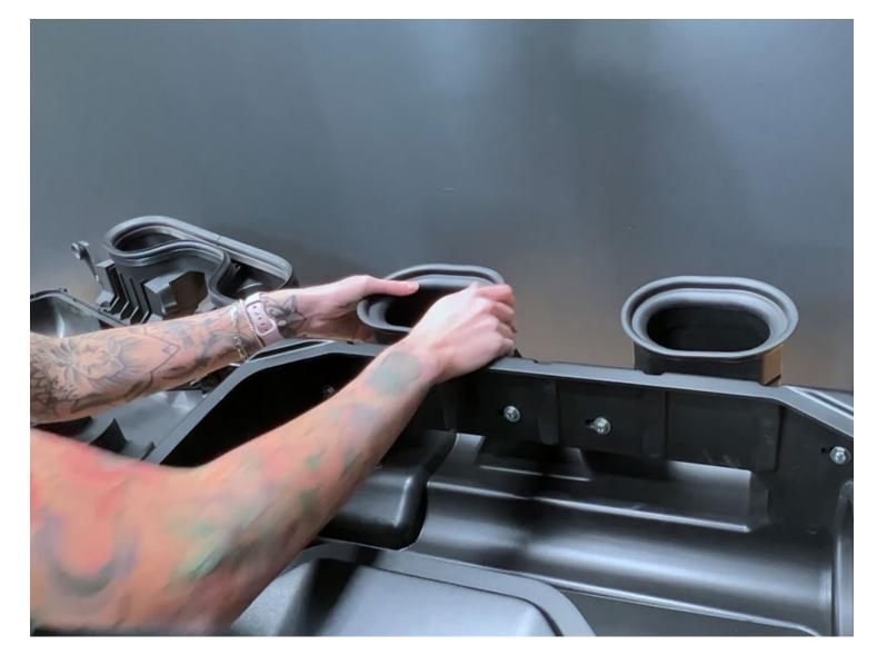
Install the silicone hood scoop seals onto the airbox.
