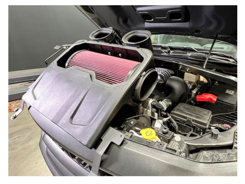
Install the airbox, support bracket, and filter assembly into the engine compartment. Push the intake tube into the filter flange and verify the S&B front airbox support brackets and the stock airbox support bracket align with their mounting holes.
