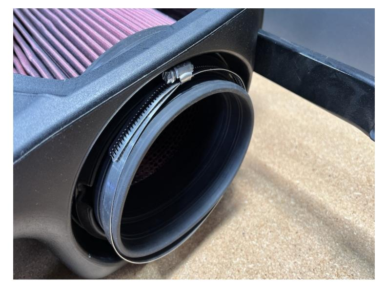
Install the hose clamp over the filter flange loosely.
