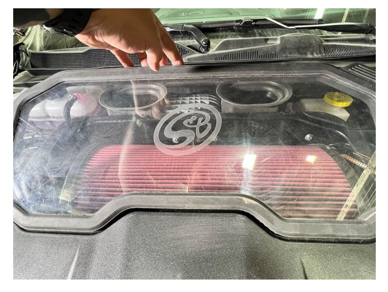
Remove the protective wrapping of the polycarbonate lid. Install the snap-in silicone lid seal around the polycarbonate lid. Install the snap-in lid assembly onto the airbox. Slide into the box as shown and use pressure around the perimeter to install the Snap-in lid.
