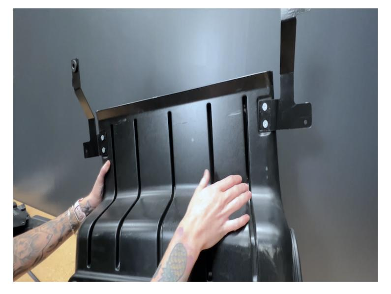
Attach the 2 airbox mounting brackets onto the front of the S&B Airbox using the supplied 1/4 -20 Torx flat head screws and a T27 Torx Bit.
