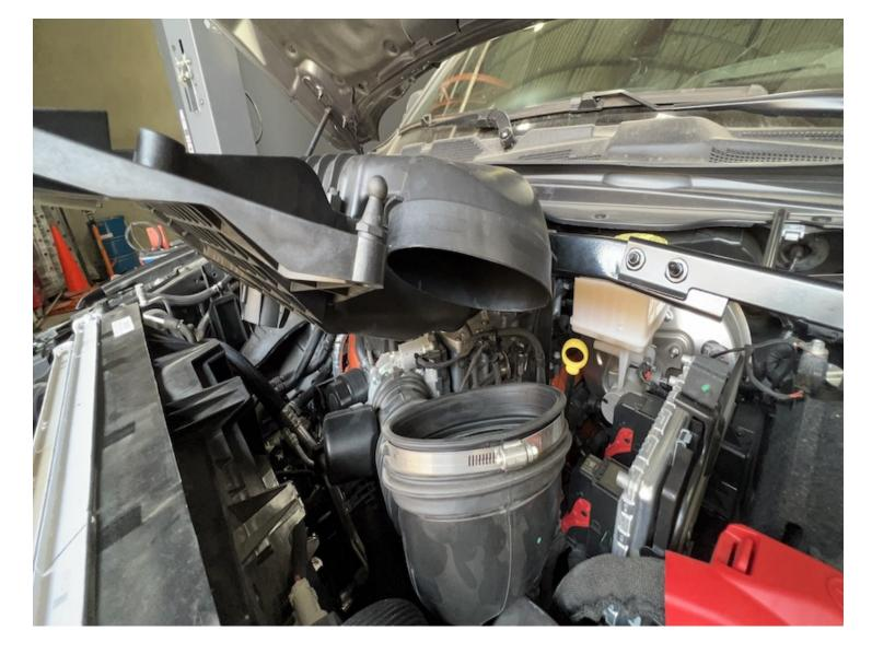
Pry up the stock airbox away from the tube and pull the airbox and support bracket assembly out of the vehicle. Set the assembly to the side.
