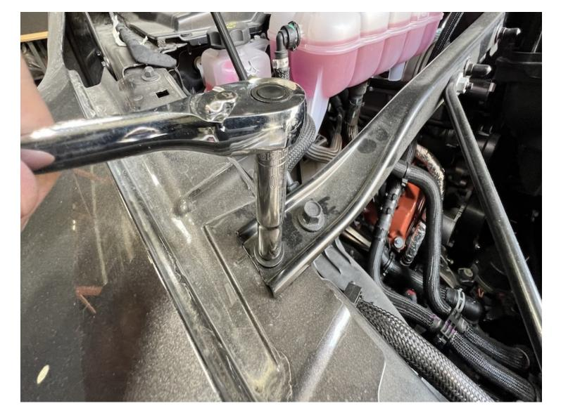
Begin removing the airbox support bracket by using a 10mm and 13mm socket at the six locations at both passenger and driver's fender sides. Collect those 6 bolts to be reused later.
