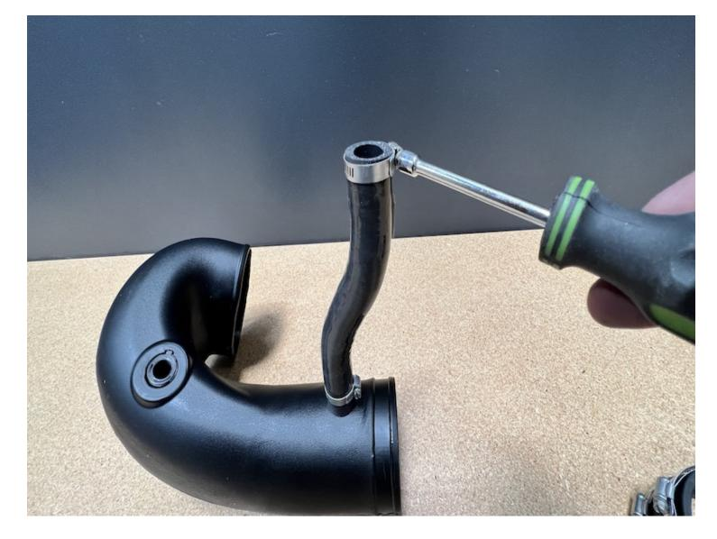
Install the CCV vent silicone-wrapped hose onto the S&B tube at the breather connection using 2 #12 hose clamps.
