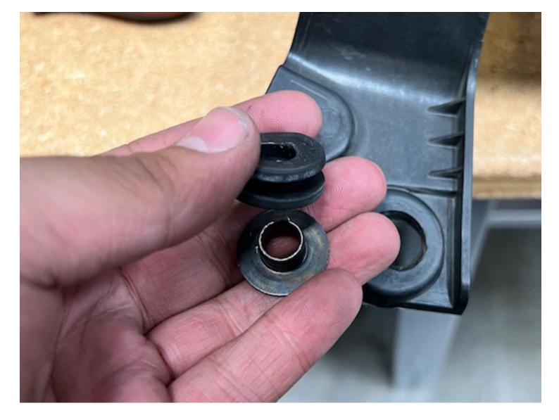
Using a flathead screwdriver pry off the grommets and shoulder spacers from the front-most area of the stock airbox.
