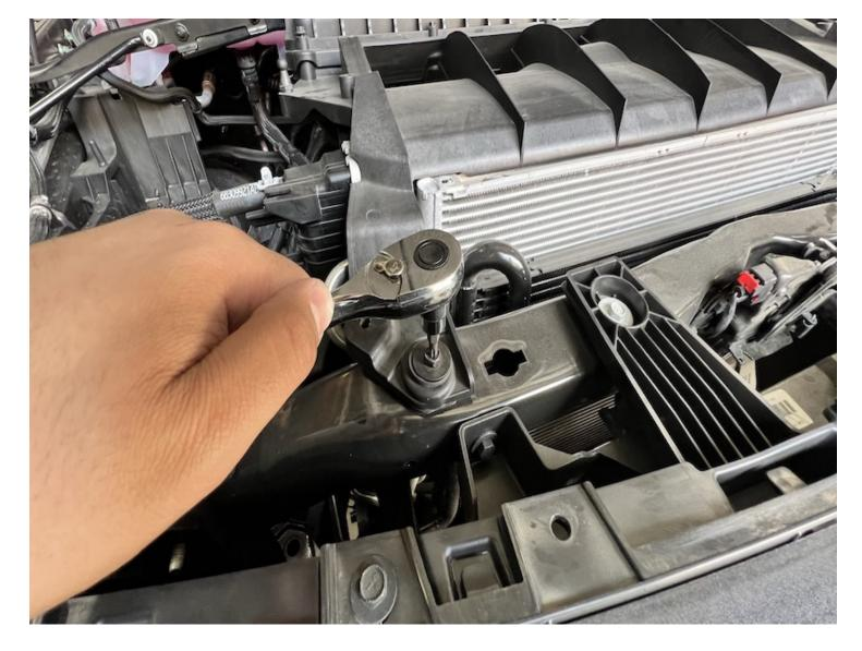
Using a T27 Torx bit or 10mm socket, unthread the 2 front screws securing the front of the airbox. Set the screws to the side to be reused later in the installation.
