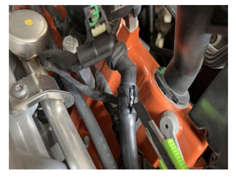
Using a knife or cutting tool, score the nylon shrink-wrapped hose at the solenoid connection. Be careful to only cut deep enough to be able to split the hose and to not cut into the plastic breather underneath. Once cut, pry the hose away from the breather.
