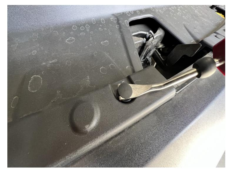
Remove the 14 reusable plastic rivets securing the radiator cover using a flathead screwdriver or panel popper. Remove the radiator cover from the engine and set it to the side. Set the rivets to the side to be used later.
