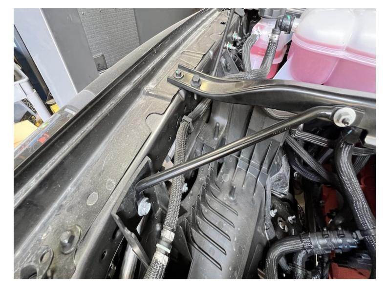
Reinstall the airbox support bracket hardware in their positions from Step 4 using 10mm and 13mm sockets.
