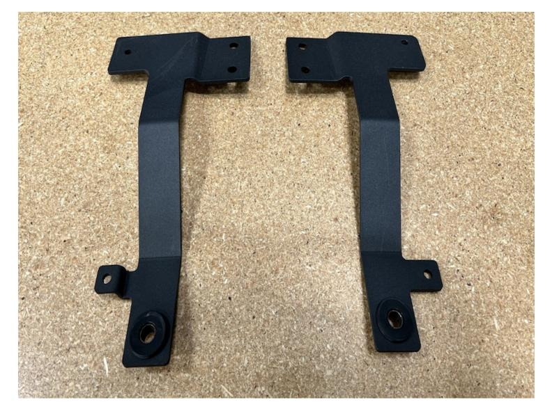
Transfer the shoulder spacers and grommets to the S&B mounting brackets in the orientation as shown with the flat of the shoulder bushing away from the scew and washer mounting area.
