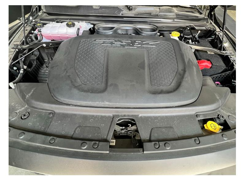
With the engine off and cooled down open the hood to begin the installation by pulling the engine cover firmly away from the stock air cleaner system.
