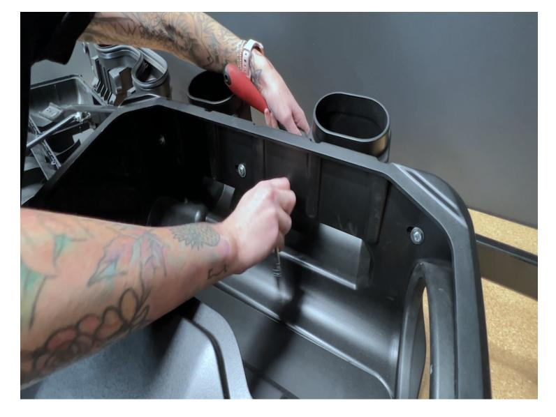
Attach the stock airbox support bracket to the back of the S&B Airbox using the provided M6 washers nuts and screws, and a 10mm socket and wrench or 2 10mm sockets. Run the screws through the S&B airbox lining up with the holes in the bracket. Do not tighten completely.
