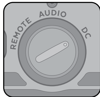
Turn Auto-Turn-On Switch to DC
