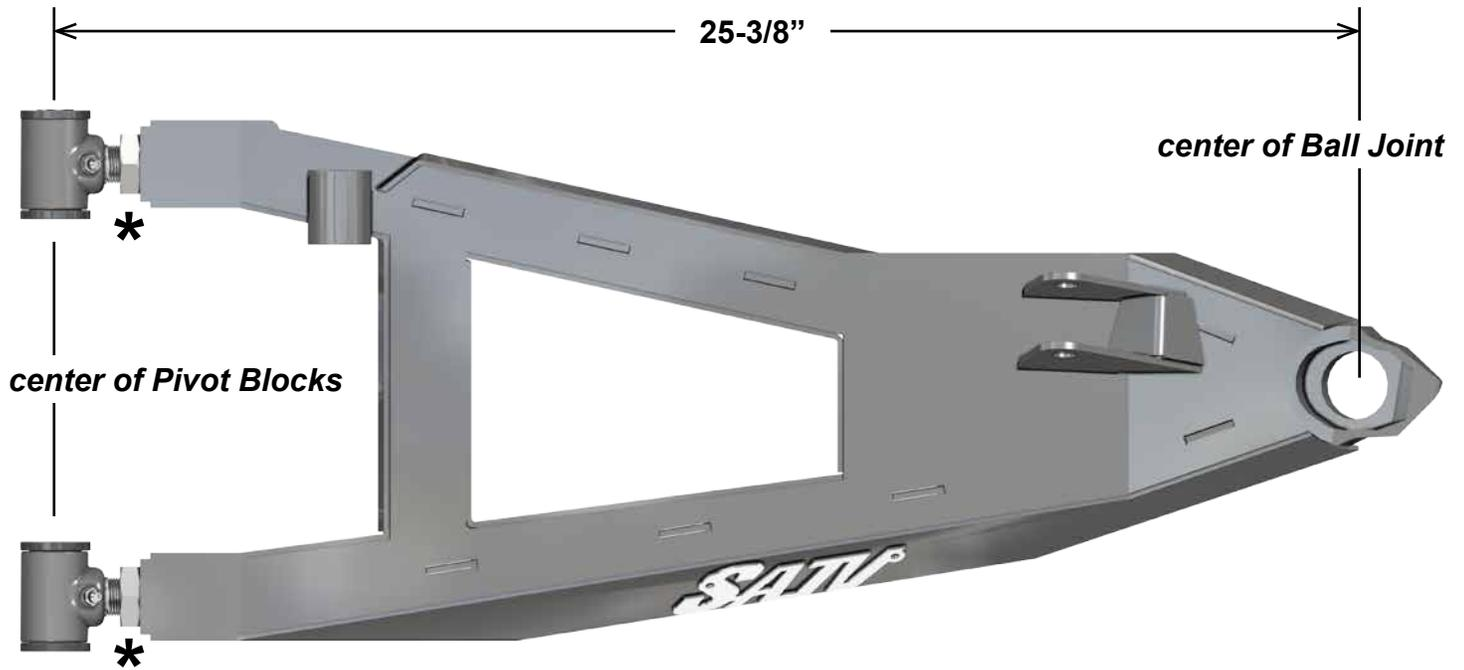
**\*Leave Jam Nuts loose. Tighten after final adjustments have been made.**
