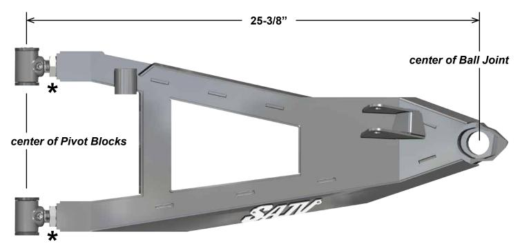
\*Leave Jam Nuts loose. Tighten after final adjustments have been made.
