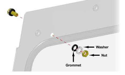
Install Wiper and Handle; do not over tighten.
