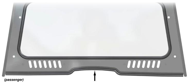
Install Seal to bottom of Frame.
