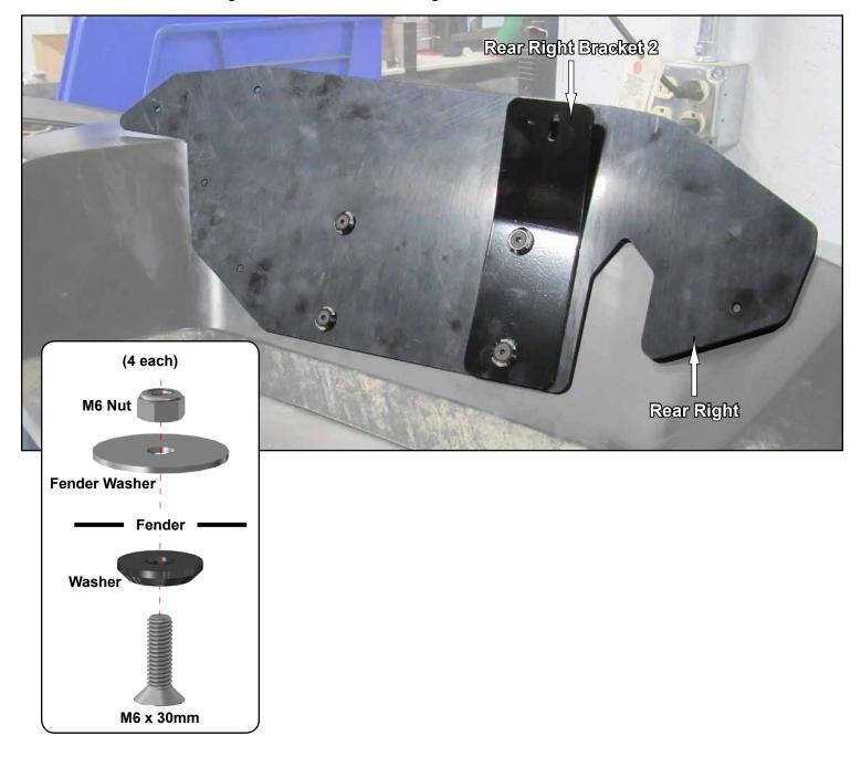
Secure Rear Right Bracket 2 and Rear Right to stock Fender with hardware shown.
