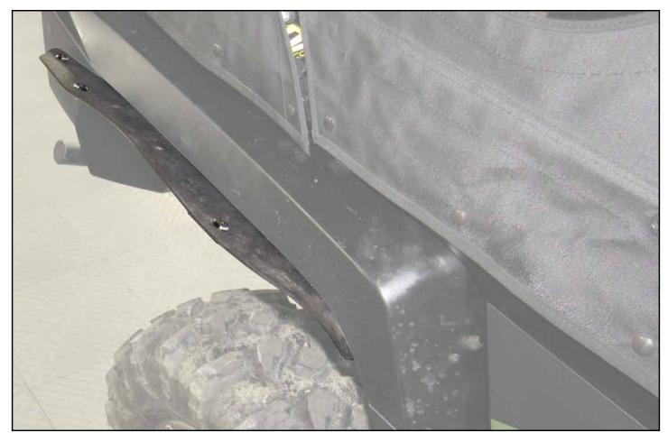
Reinstall stock Fender with stock hardware.
