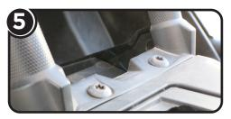
Next, remove the bottom 2 torx T-30 bolts in between the console pillars.
