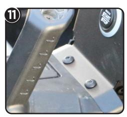
Attach Start/Stop button. Reinstall the Torx Screws removed in step 2 and install the bolts into the  $\frac{1}{4}$ " drilled holes from step 6 and secure.
