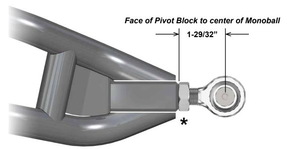
\*Leave Jam Nut loose. Tighten after final adjustments have been made.
