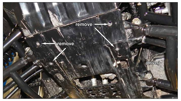
*do not tighten any hardware completely unless noted* - Install Plate (A) to machine with hardware shown.
