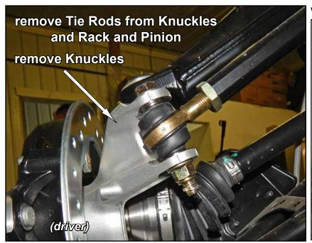
Tip: rotate Knuckle and use setup shown when removing/installing from Upper Arm.
