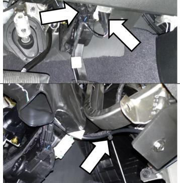
Use the supplied alcohol wipe to clean the surface where the TSBooster will mount. Apply the double-sided tape to the chosen mounting location (trim tape to length if needed). TOTAL TOTAL
