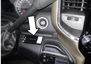
Turn the ignition switch to the on/run position but don't start the engine.
