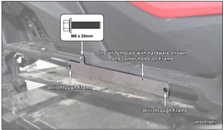
remove Template and reinstall stock Screw
