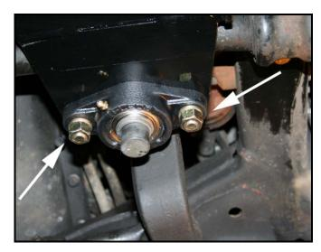
Remove the set screws and apply LocTite.
