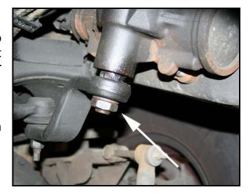
A 1-1/4" deep socket (180 lbs-ft) should be used to install the new sector shaft nut, re-using the stock lock washer.
