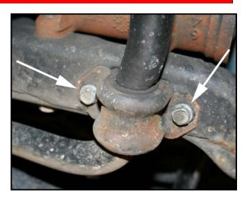
Allow the sway bar to swing down and rest onto the steering linkage.
