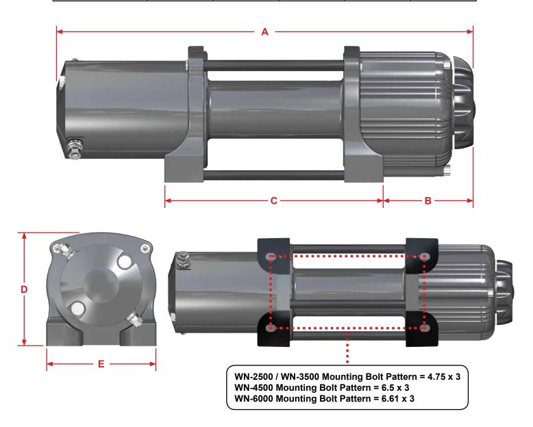
**WN-2500:** Synthetic Rope (Diameter x Length): Ø3/16" x 50' (Ø4.8mm x 15.2m) **WN-3500:** Synthetic Rope (Diameter x Length): Ø7/32" x 50' (Ø5.5mm x 15.2m) **WN-4500:** Synthetic Rope (Diameter x Length): Ø1/4" x 50' (Ø6.3mm x 15.2m) **WN-6000:** Synthetic Rope (Diameter x Length): Ø17/64" x 50' (Ø6.6mm x 15.2m)
