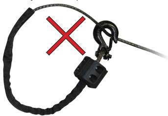
CAUTION - Use Hand Strap when handling Clevis Hook. Use gloves to protect hands when handling Synthetic Rope. Never let Synthetic Rope slide through bare hands.
