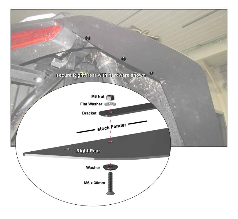
use a Ø1/4" bit and drill holes into stock Fender
