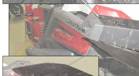
Rivet - use a Ø1/4" bit and drill hole into stock Fender - secure Right Rear with hardware shown
