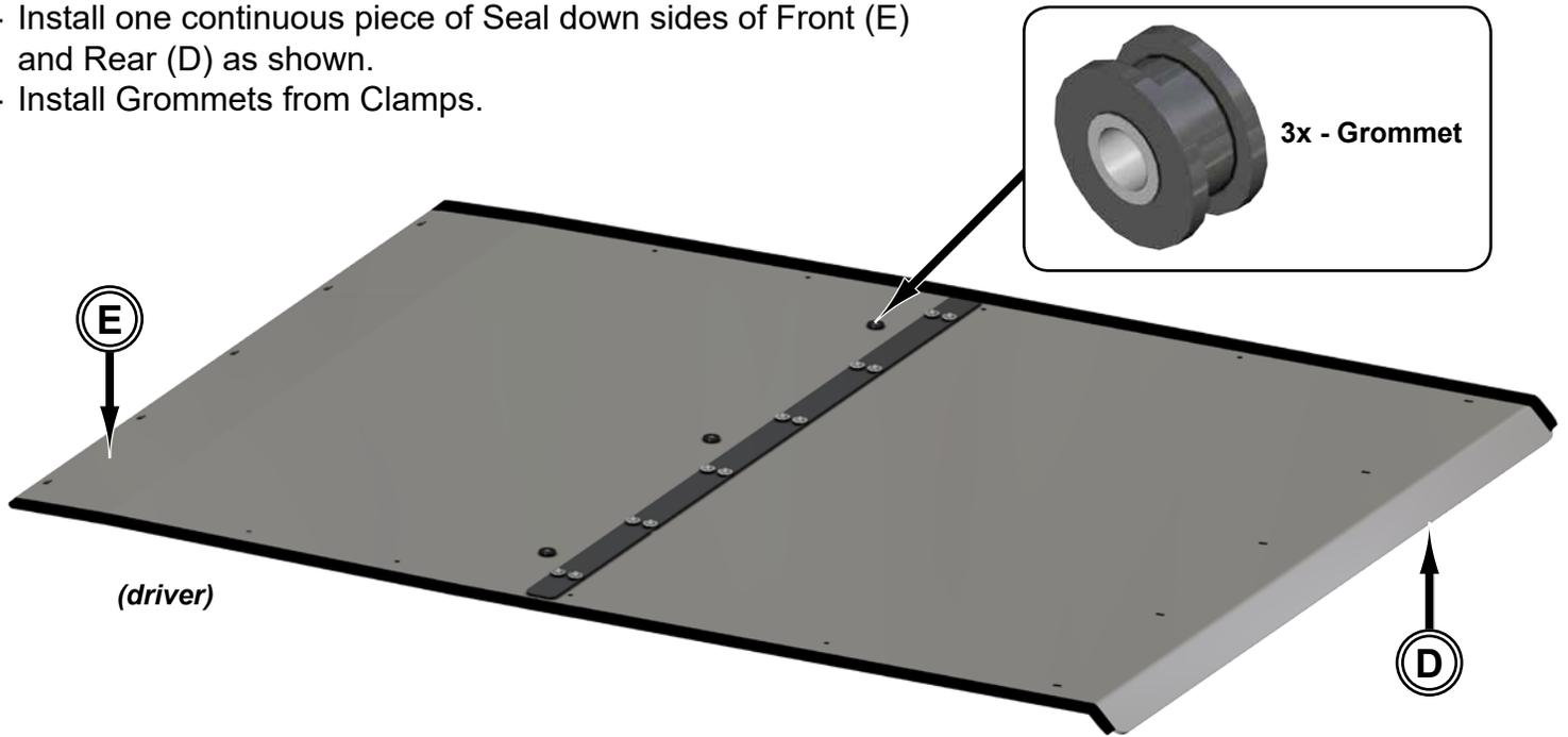
**Soak Seal in hot water before cutting or installing to increase flexibility.**
