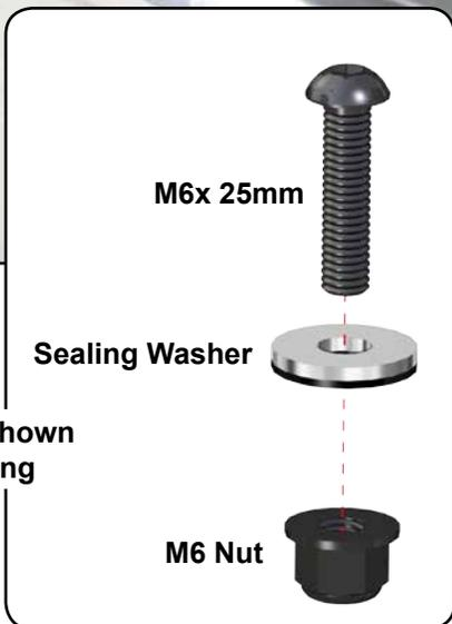
**tighten hardware completely**
