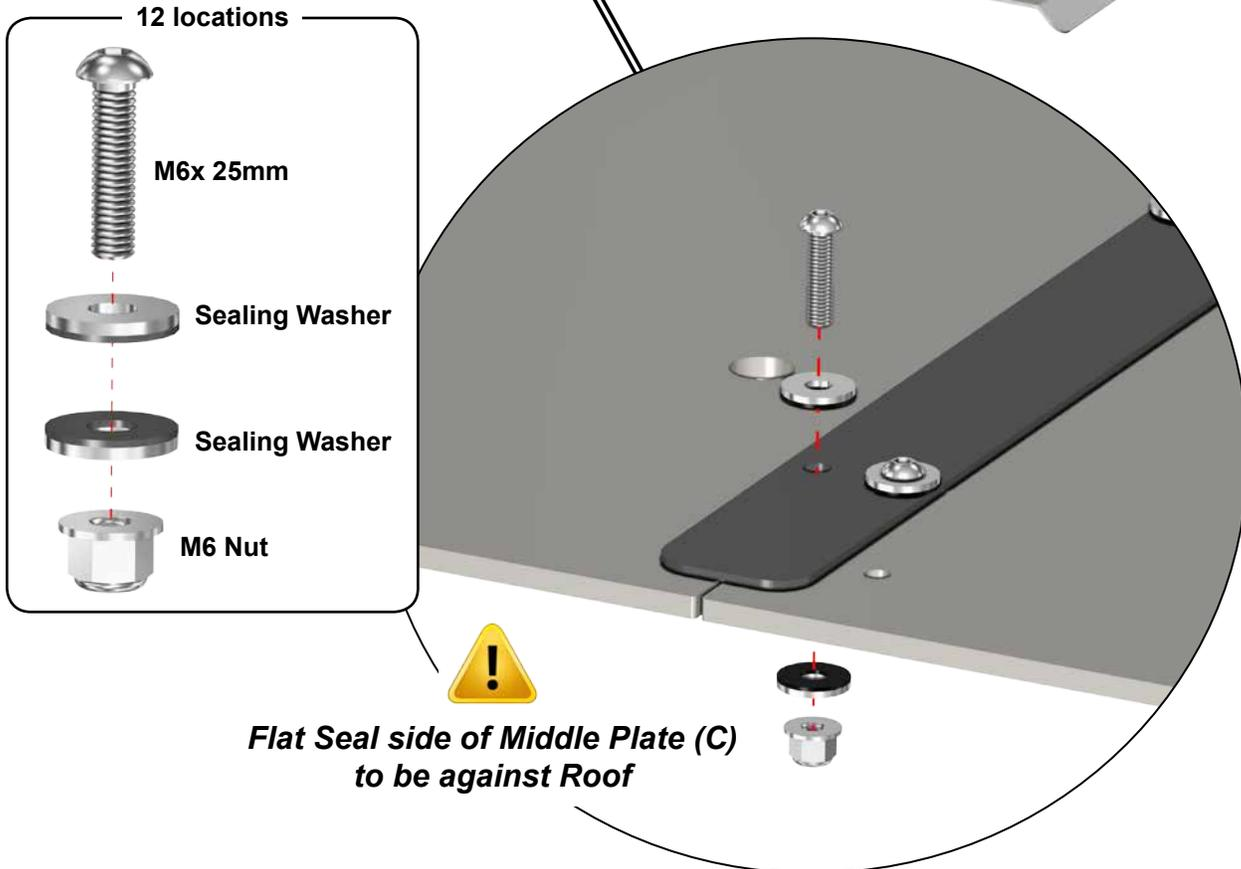
**tighten hardware completely**
