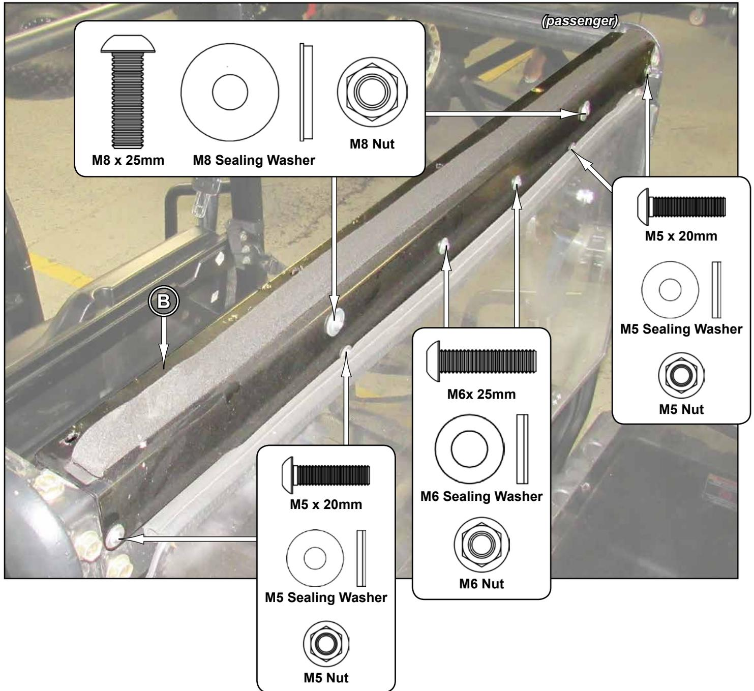
**tighten hardware completely**
