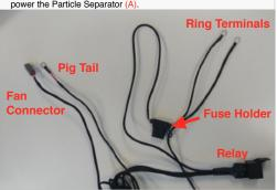
$\bf 31.$  Install the ring terminals onto the battery terminal clamps. Red wire with the fuse holder to (+) and Black wire to (-). Secure the positive terminal first and then secure the negative terminal
