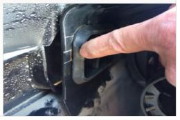
11. Reinstall the stock foam air cleaner element.
