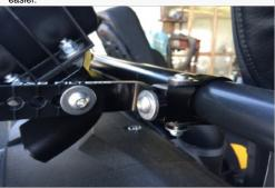
23. Once you are satisfied with the position, use a 4mm Hex Key and 10mm wrench to tighten the Screw (J), Washer (I), Locknut (K) at the Strap (H).Do this for both sides. Go over all the screws and locknuts again to make sure they are secure and that the Particle Separator (F) is firmly attached to the roll cage.
