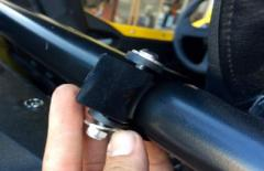
20. Use a 13mm wrench and 5mm Hex Key to install the Adapter (B) onto the bottom of the Particle Separator (A) with the supplied Screws (D), Washer (C) and Locknuts (E). Tighten these screws and locknuts.
