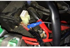
$38.\,$  Find Fan Connector and connect it to the Particle Separator (A). Make sure not to cross the connectors. Power to power and ground (black) to ground (black). Note the color of the wires whenever connecting or disconnecting this connector. The connector should snap into each other with very little resistance. Do not try to force the connectors into each other.
