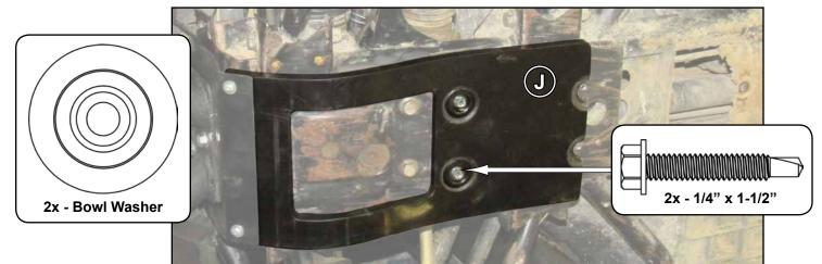
install Front Metal Plate (A) to Front Plate (J) and Frame with hardware shown
