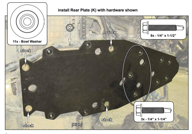
Rear Spacer (L) goes between Rear Plate (K) and Frame
