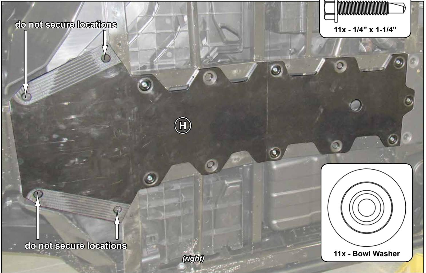
install Front Plate (J) with hardware shown
