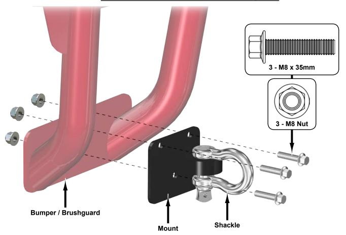
Do not tighten hardware completely unless noted.
