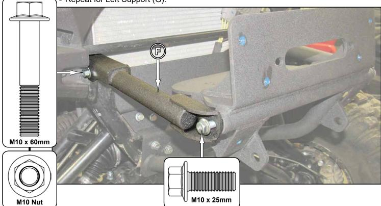
Install Winch at this time and tighten all hardware completely.
