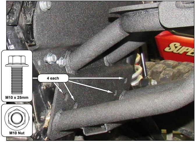
Install Right Support (F) to Frame and Mount Plate (B) with hardware shown.
