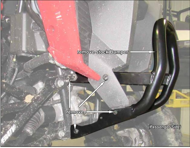
Do not tighten any hardware completely unless noted.
